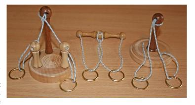
John produced a thick bar-bell shape with parallel small holes to take the string through the spheres and the ends and at right angles an 8mm hole in the centre. Decorating and finishing the piece John then tied the string and rings to the piece as shown in the puzzle in the centre of the
